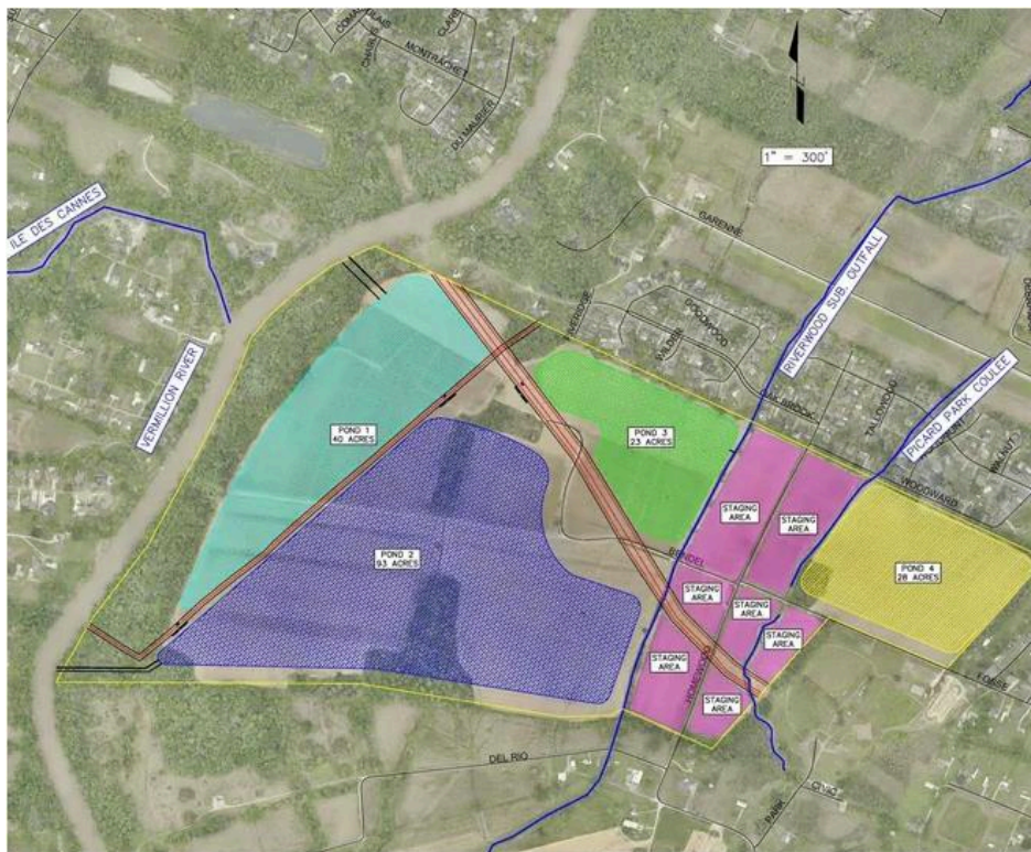
Preliminary designs by McBade Engineers, who LCG has contracted for its $35 million Homewood Detention Project, show several ponds intended to lower water levels on the Vermilion River in Lafayette. Courtesy Of Lafayette Consolidated Government
